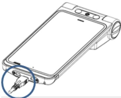
1. Connect power supply for the first time and make sure battery is fully charged before disconnecting.
